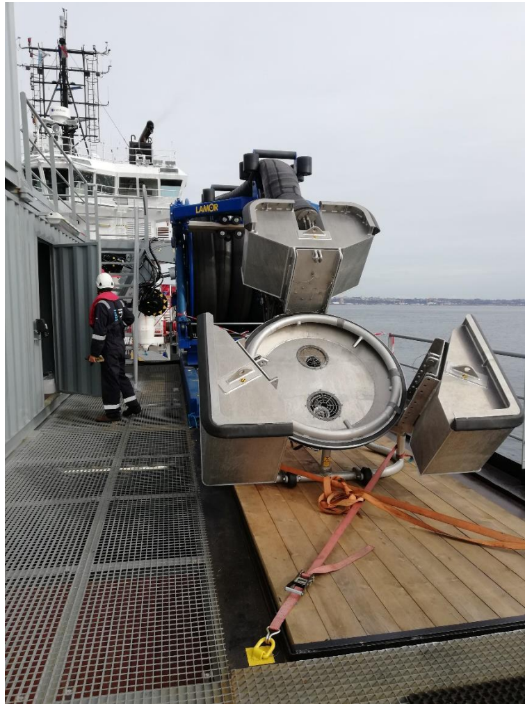
Fig. 18. Lamor Free Floating High Capacity Offshore Skimmer weir module
