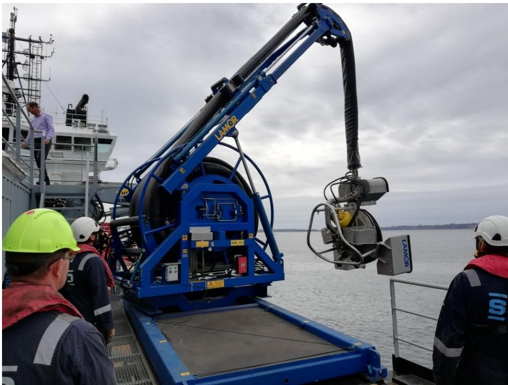
Fig. 14. Umbilical Hose Reel LUT 90, with Telescopic Crane Arm
